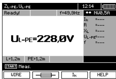
Checking effectiveness of protection against electric shock of the housing in case of: a) TN b) TT.
